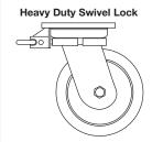
This husky, plunger-type swivel lock, with cast malleable iron body can be welded to any of the heavy-duty casters.
